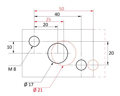
Dimensions in red with spindle diameter 20 mm Dimensions in black with spindle diameter 16 mm
